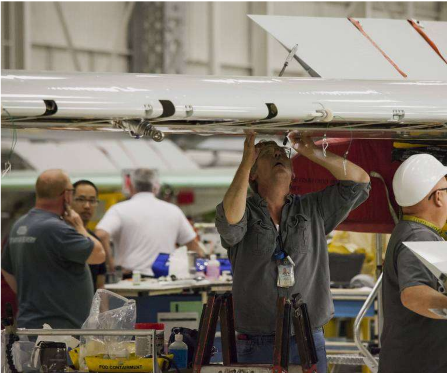
Employees install panels on airplane wings at the Boeing Co. manufacturing facility in Renton, Wash., last year. PHOTO: DAVID RYDER/BLOOMBERG NEWS
