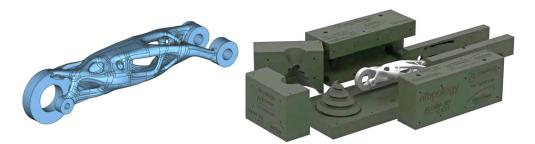
Humtown, nTopology, Penn State, Jarvie Performance Castings and Flow 3D Cast created an end-to-end digital sand casting work flow to create a topology optomized robot arm that was over 1 meter in length and and weighs over 240 pounds.
